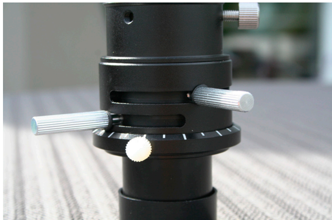
Fig. 2: The small white screw marks the zero scale position. The levers are moved in opposite directions.
