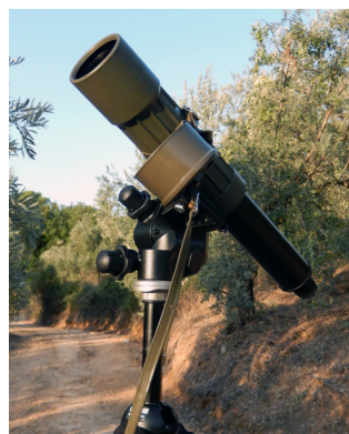
Figure 10: 75/524 mm refractor, mounted on a Manfrotto 055 Pro tripod with 410 Junior Geared Head.
