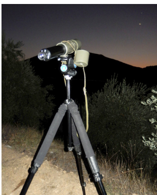
Figure 9: 75/524 mm refractor (30x magnification), mounted on a Manfrotto 055 Pro tripod with 410 Junior Geared Head, the latter offering precise geared movement in three directions. Moon and Venus are seen on the upper right.
