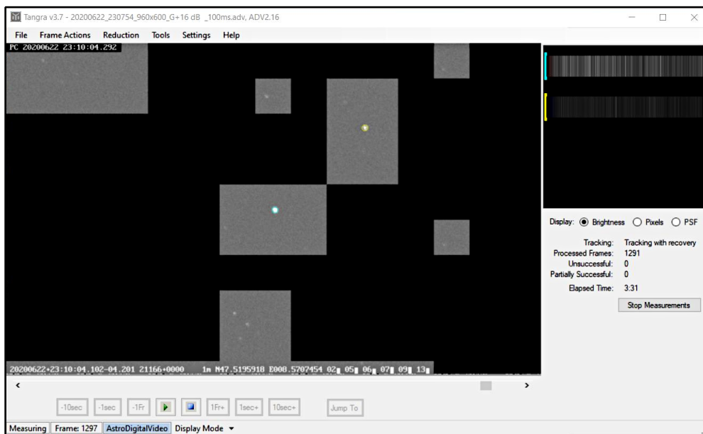
Figure 2b. The ROI-only ADV file displayed in Tangra. Only the pixels in the selected ROIs are actually saved in the ADV video recording.
