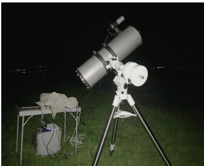
Figure 2. Photo of the 203/810 mm Newtonian telescope observing a positive occultation of the asteroid (893) Leopoldina on 2020 July 1 over the Danube Valley in Lower Austria.
