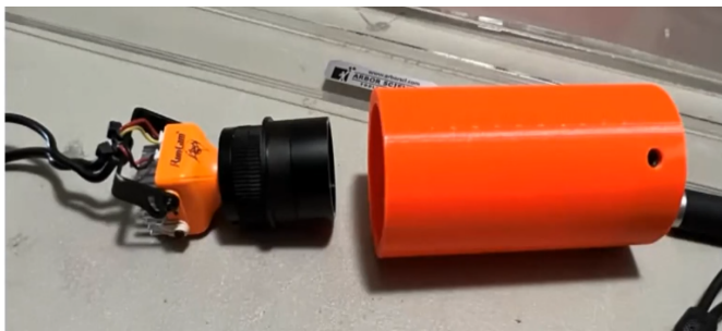
Figure 7. 3D-printed carrier for the Run Cam Eagle (left).
