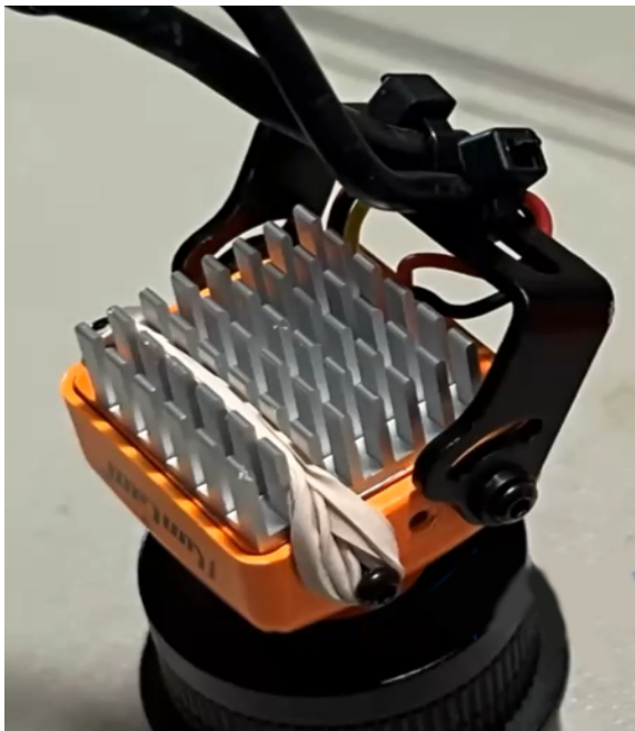
Figure 8. Heat sink mounted on the camera.
