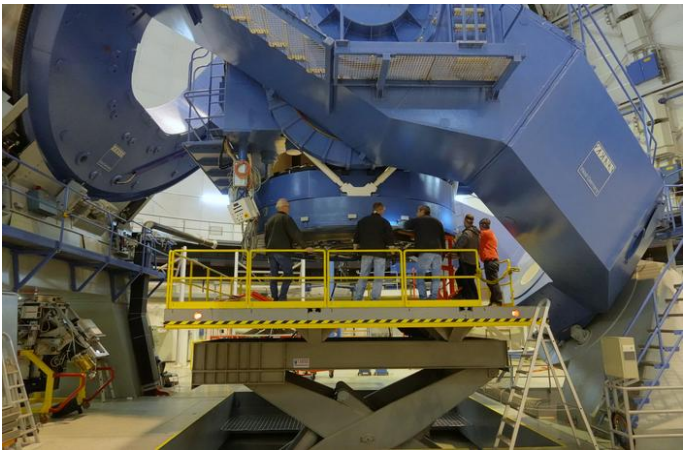
Figure 14, 15. The technicians are ready to remove the primary mirror of the 3.5-m telescope. (O. Klös)
