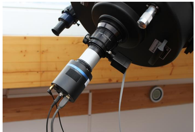
Figure 6. QHY 174M-GPS camera mounted on the telescope, the reducer is inside the draw tube.
