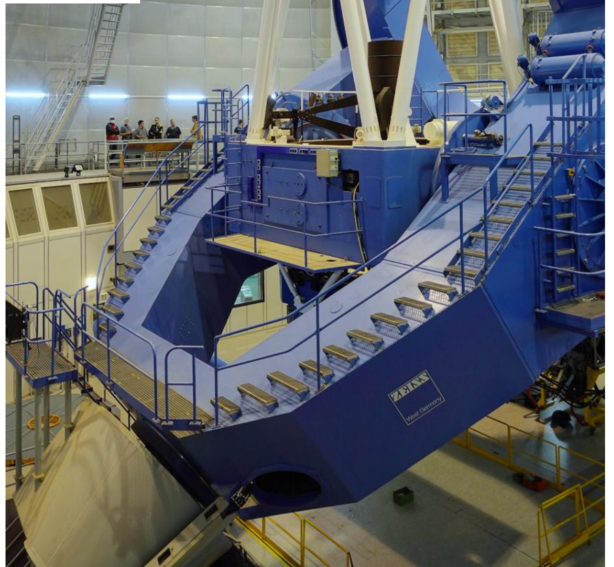
Figure 14, 15. The technicians are ready to remove the primary mirror of the 3.5-m telescope. (O. Klös)
