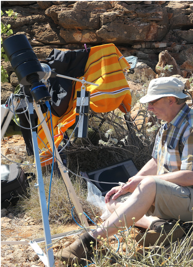
Figure 3. The author at the set-up station with 100/1000 Maksutov on a travel mount and a camera QHY174M-GPS. In his hand the control-box for the fine adjustment of the drive of the mount, on the monitor the Sun as a crescent. (Photo: Elke Guhl)
