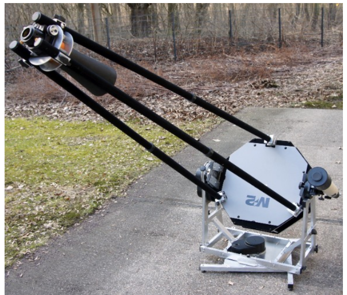
Figure 13. The IOTA/ES M2 telescope with a diameter of 50 cm. (K. Guhl)
