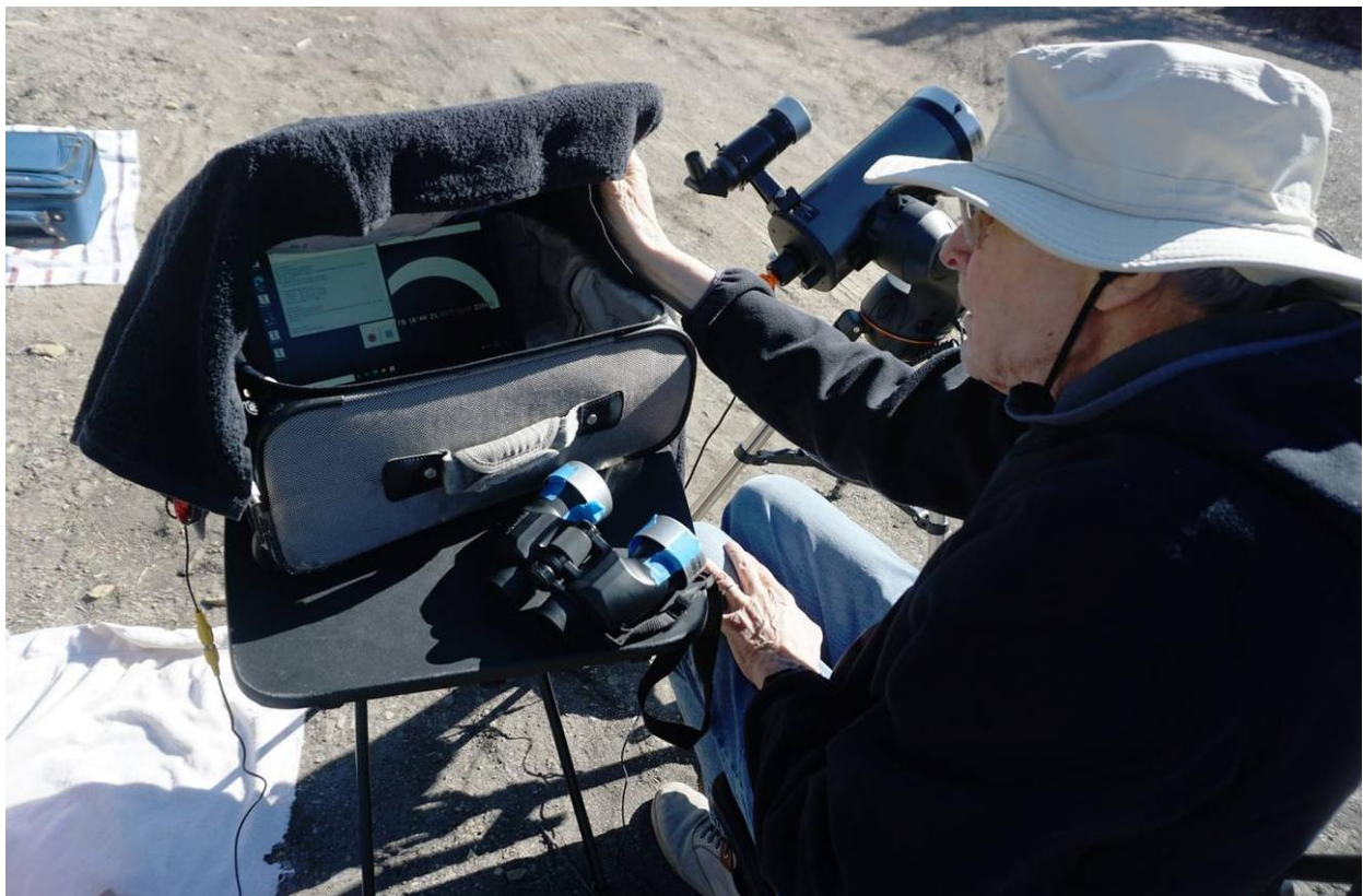
Figure 3. Laptop displaying video. The laptop is shielded from the Sun in a small carry-on suitcase with the aid of a black towel.
