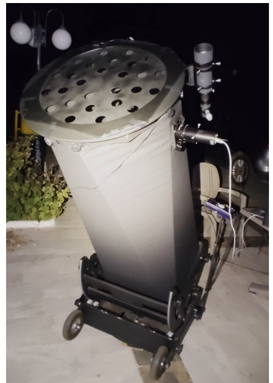
Figure 5. Noschese's "Leviathan" 50 cm Dobsonian telescope with mask. (A. Noschese)
