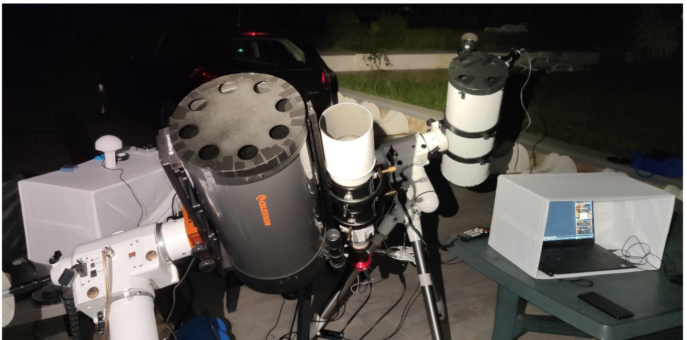
Figure 7. The telescopes' setup at Noschese's observing place: C9 and 10 cm refractor. (A. Noschese)
